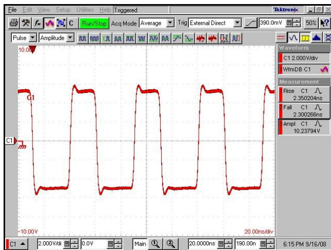
Figure 1. Pulse Output at 20MHz Repetition Rate, 2ns Rise/Falltime, 20ns Pulse Width, and 10V pp
