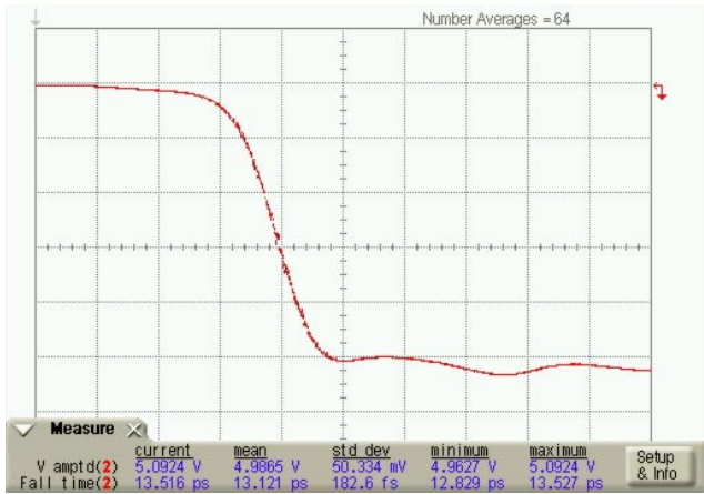
PSPL 4015D Pulse Generator Step Output and Resulting Impulse Using the 5206 Impulse Forming Network
