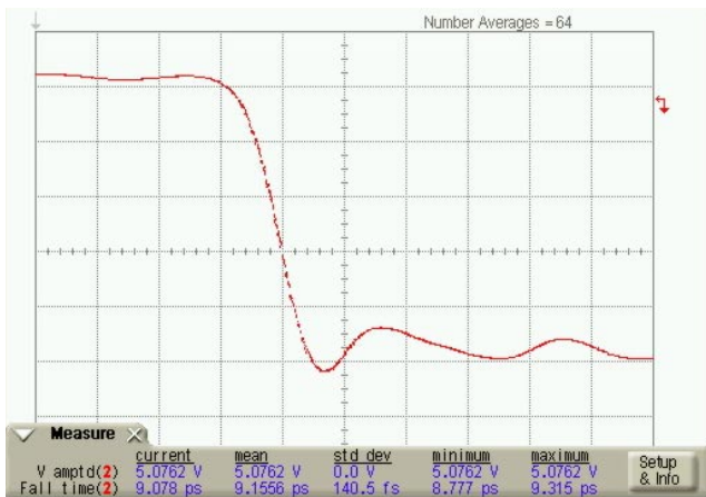
PSPL 4016 Pulse Generator Step Output and Resulting Impulse Using the 5206 Impulse Forming Network
