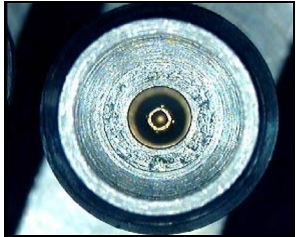
Figure 3. Damaged Female Connector
