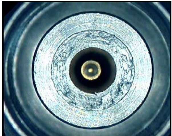
Figure 5. Damaged Male Connector
